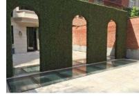
A new system of walkable skylights called SkyFloor from Glass Flooring Systems can be used in pedestal paver applications. The system features thermally broken frames, fully independent structural framing and extruded aluminum structural rafters. Standard and custom sizes are available for the system, which can include various anti-slip tested surfaces and integrated LED lighting. The stepped design frame transfers the load of the structural floor glazing off the insulating glass unit.
